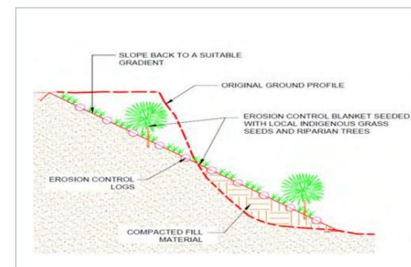
Figure 18: A diagram showing how sloping and revegetation is typically set out
