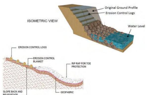
Figure 9: Diagrams showing how rip rap and sloping is typically set out
