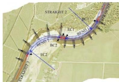
Figure 26 showing typical layout of groynes in relation to river geometry
