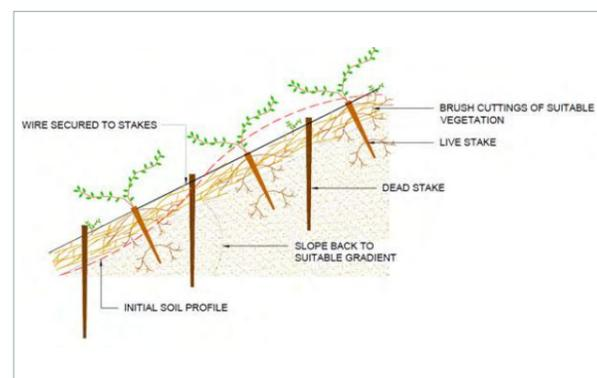
Figure 10: A diagram showing how brush packing is typically set out
