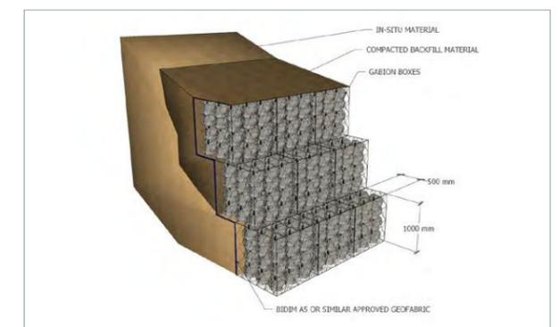
Figure 22 showing typical riverbank design of gabion bank protection
