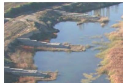
Figure 25 showing oblique aerial view of groynes as riverbank protection
