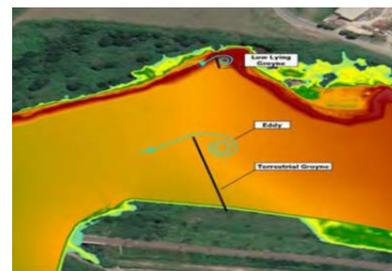
Figure 27 showing hydraulic model of river after groyne construction.
