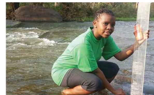
Figure 37. The velocity plank can be used to determine flow velocity of a stream, as well as depth and discharge (The Water Wheel, 2018)
