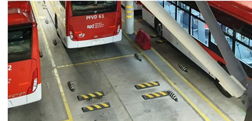
Figure 16. Stopping points on the floor of a bus depot inform the driver they have reached the desired stopping location.
